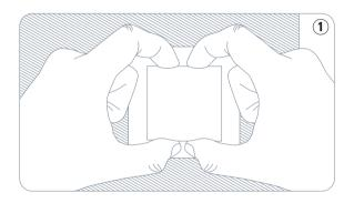
2 Press both left buttons simultaneously for 10 seconds.
