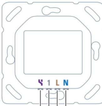
External Input      Output      Outer conductor/Phase      Neutral
