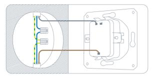
Remember which line is connected to the input on your old light switch (L), for example by marking it with adhesive tape. Then disconnect the existing wiring and remove your old light switch.
