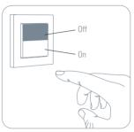
If you have mounted Eve Light Switch the other way around, you can flip the on and off orientation in the accessory settings.
