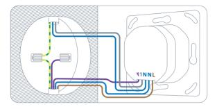
Eve Light Switch does not require a connection to a protective conductor / ground wire (PE, usually green/yellow).
