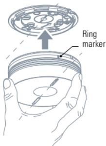
Applying gentle pressure, press and turn Eve Smoke in a clockwise direction until it locks in place.
